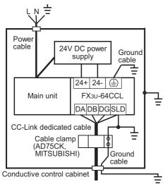
· Wiring simplified diagram
